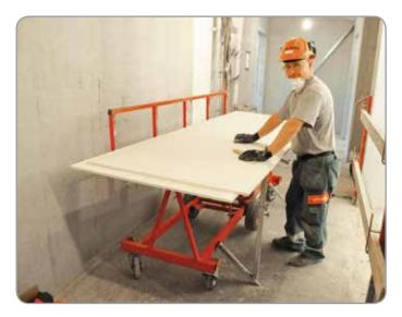
Transport mode using the pneumatic wheels for easy rolling over rough surfaces.
